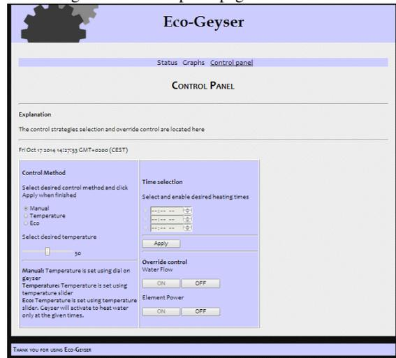
In the Temperature control scheme, the control module cuts power to the element when it reaches a desired temperature. The user can set the desired temperature on the interface.
