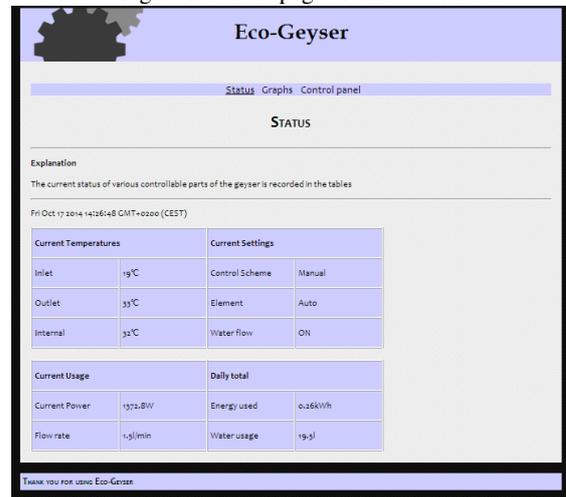
The status page was designed to give the user an indication of the most important parameters of the intelligent water heater system at a glance. These parameters are current values being measured and the active control scheme. The three temperature measurements, current water and power usage and daily totals for water and energy usage are given. This page can be seen in figure 2.
