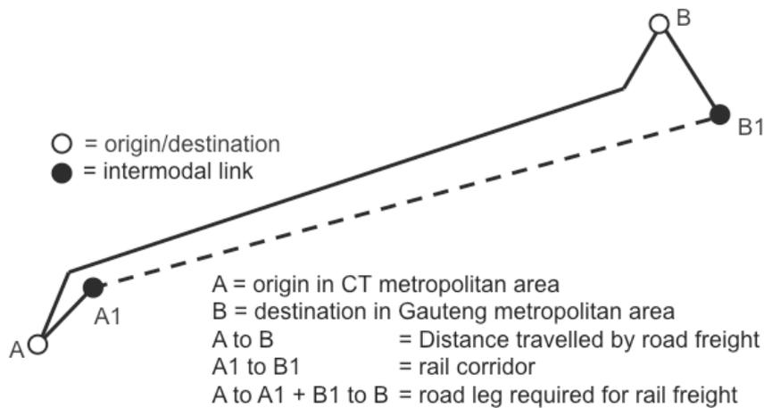
**Figure 3: Routes modelled for transport of freight by road and rail**
